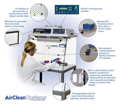
Both types of cabinets are available in two sizes and incorporate the following features:
