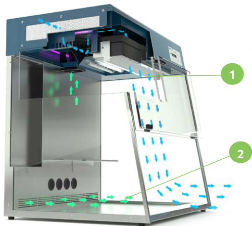
Workstation in operation mode 1. Visualization of the air flows inside the HEPA workstation with fresh air intake (blue arrows) 2. UV air recirculator (green arrows)
