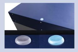
Indicator for UV Air Recirculator tube at the back upper side of the device for control of proper function.
